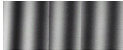
Fig. 2 Interferogram with carrier fringes.
