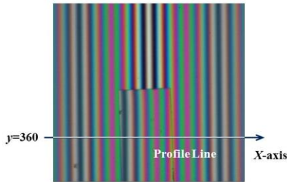
Fig.4 Color image of 1 \mu\text{m} step height (512×480pixel)
