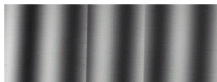
Fig. 2 Interferogram with carrier fringes
